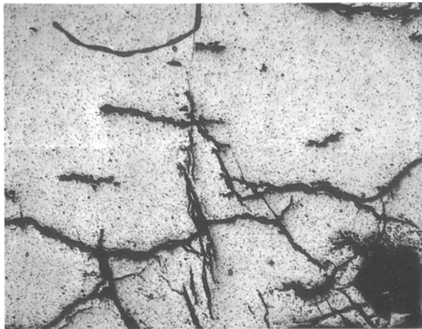
Figure 10 Optical micrograph of cracked area of sample sintered at 1750°C from shock compacted ( 871 \text{ m sec}^{-1} ) powder. (14 ×).
